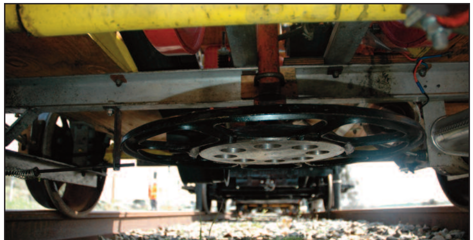
A rod from the side of the car serves as the safety lock. The hydraulic cylinder is mounted to the frame member in the center of the car. A boxcar brake wheel (with some modifications) serves as the turntable foot. Photos by Wayne Parsons
